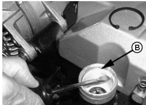
Remove Thermostat (Later Engine Shown)
