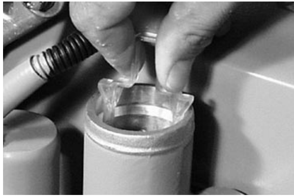
Removing Thermostat from Housing (Earlier Engine Shown)
