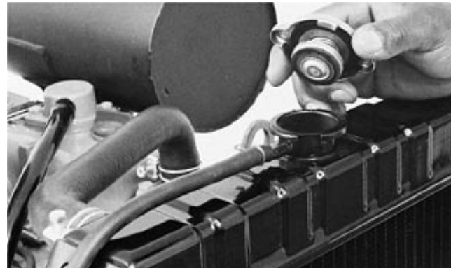
Check Coolant Level in Radiator
