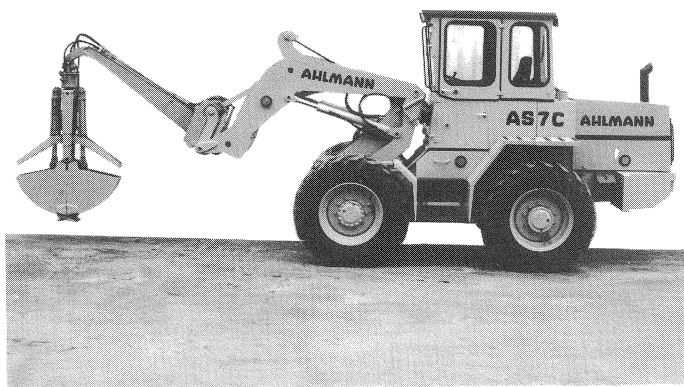
Fig. 4 Swing shovel loader with grab
