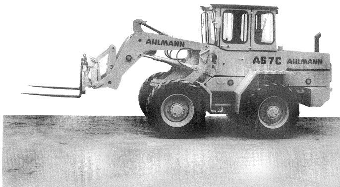
Fig. 7 Swing shovel loader with fork-lift attachment
