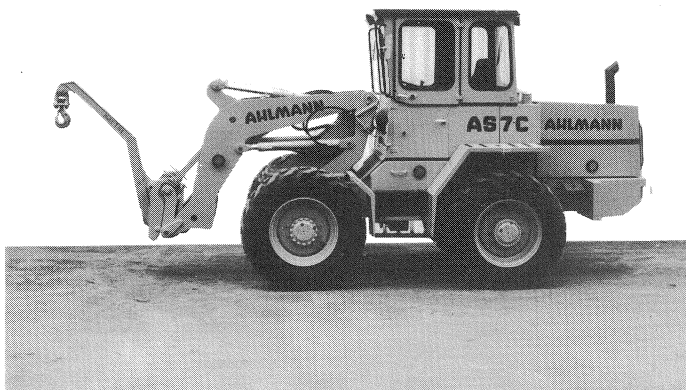
Fig. 6 Swing shovel loader with crane hook
