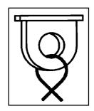
Ball block valve for working/auxiliary hydraulics closed
