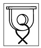
Ball block valve for working/auxiliary hydraulics closed
