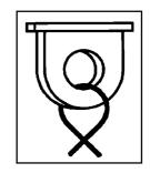
Ball block valve for working/auxiliary hydraulics closed
