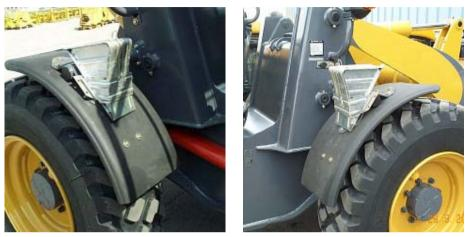
The wheel chocks are housed in two supports located on the front mudguards of the vehicle.
