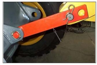
**Stage 1** Insert the locking rod for bucket and loader booms.
