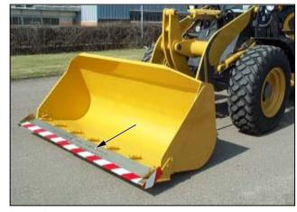
Stage 2 Install the loader bucket teeth-protection.
