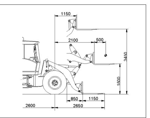
Load 2,600 kg. (with quick coupling 2,400 kg)
