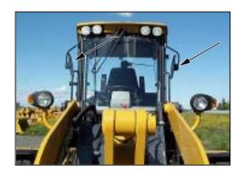
Stage 5 Turn the rear view mirrors inwards and make sure that the two doors and the rear cab window are closed.
