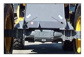
If the vehicle must be towed due to malfunction, use a fixed bar suited to its weight fastened to the tow flaps located at the front of the vehicle. (see photo).
