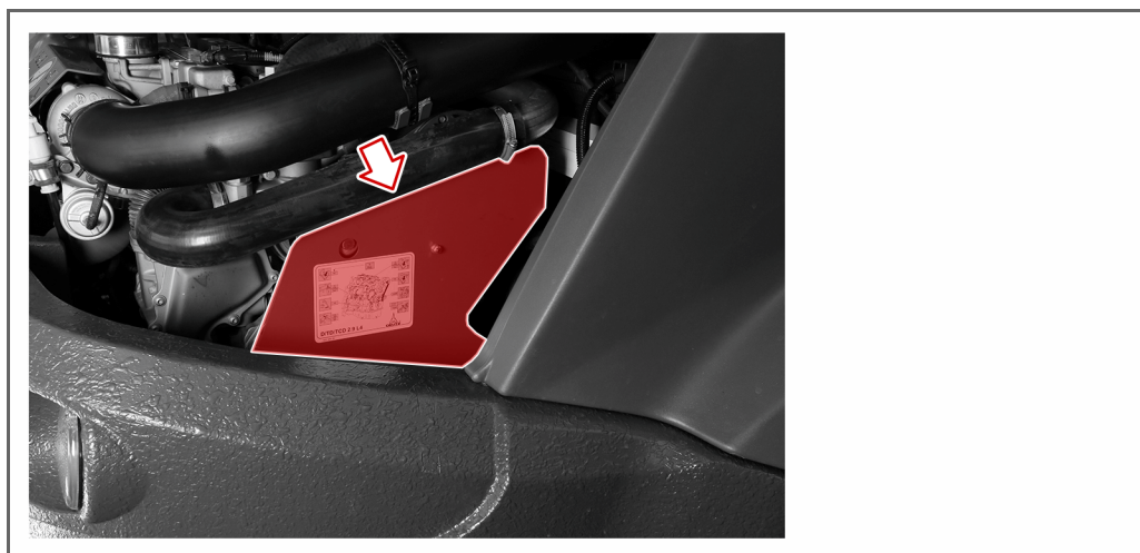
Location of the V-belt guard plate
